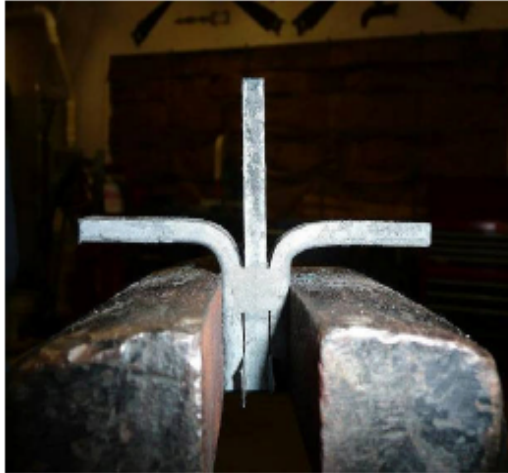
Figure 2: Blank after first set of bends, notice the spacers (left), finished snowflake (right)
